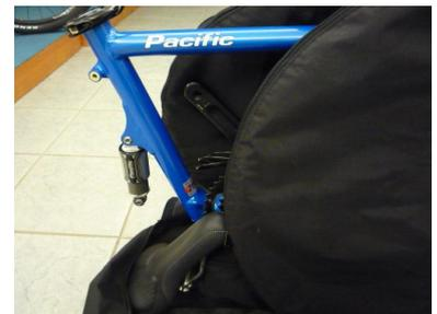
13 將攜車袋兩邊拉鍊拉上；[束帶]穿過攜車袋孔位、車架上管,並束至最緊
